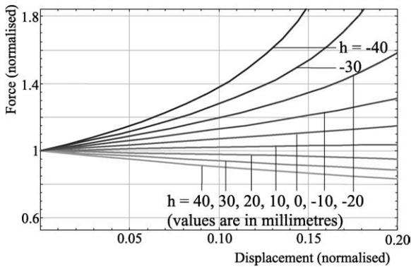
Fig. 5. The force–displacement curves shown here with varying  $h$  values suggests that low resonant frequencies can theoretically be achieved by this spring coefficient reduction technique. In reality, the performance of the springs only benefit when operating at small spring buckling deflections (to about 3% of their unbuckled length).
