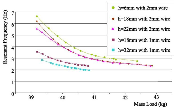
Fig. 9. Plot of the resonant frequency as a function of mass in the Euler stage with different values of the inverse pendulum height  $h$ . The distinct different operating ranges in mass load between the different sized wires clearly suggests the system with the 1 mm wire is softer.
