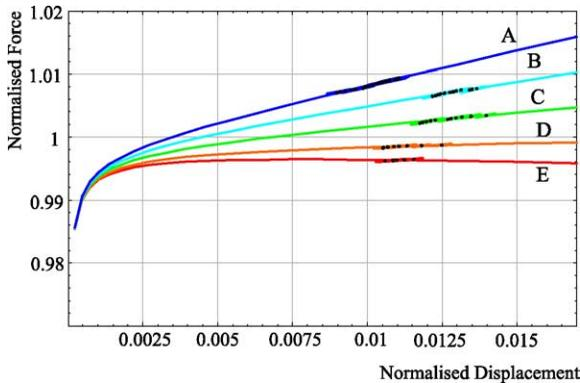
Fig. 10. The force–displacement curves for experimental launch angle  $\theta = -0.0225$  radians (adjusted to  $-0.00070$  rads), (A)  $h = 45$  mm, (B)  $h = 55$  mm, (C)  $h = 65$  mm, (D)  $h = 75$  mm, and (E)  $h = 81$  mm.
