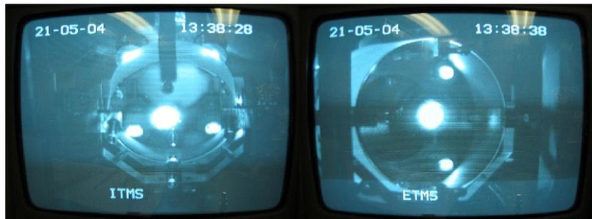
**Figure 6.** The pictures show the images from the CCD cameras mounted outside the vacuum tanks. The cameras are used to monitor the test masses during locking and operation. We can see the cavity locked and the fundamental mode reflected in both test masses.
