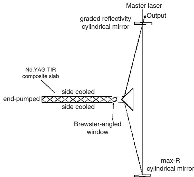
**Figure 1.** Schematic of the high power slave laser. The resonator is unstable in the direction perpendicular to the page and stable in the orthogonal direction.
