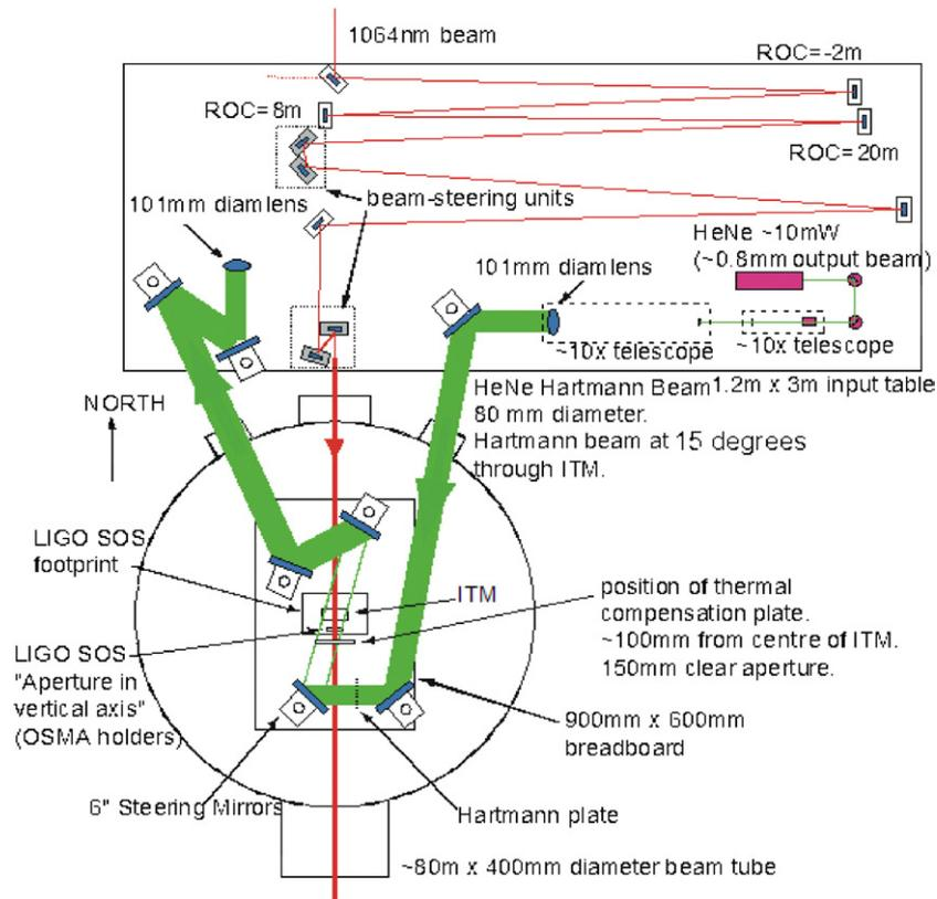
**Figure 3.** Schematic diagram that shows the distribution of the input test bench including the ITM and the Hartmann sensor inside the vacuum tank.
