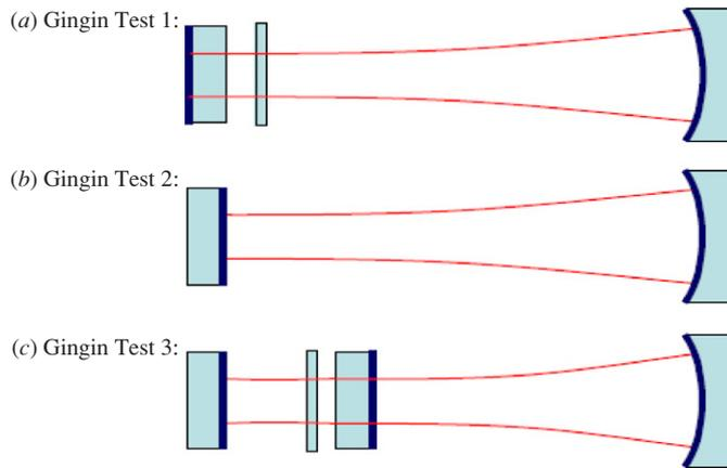
**Figure 4.** Gingin tests are designed with different purposes. Test 1 is to quantify and correct thermal lensing effects using two sapphire test masses and a fused silica compensation plate. Test 2 will use the same test masses to study thermal effects in the HR coating. Test 3 includes a fused silica power recycling mirror to increase the power in the cavity for further study of thermal effects and radiation pressure.
