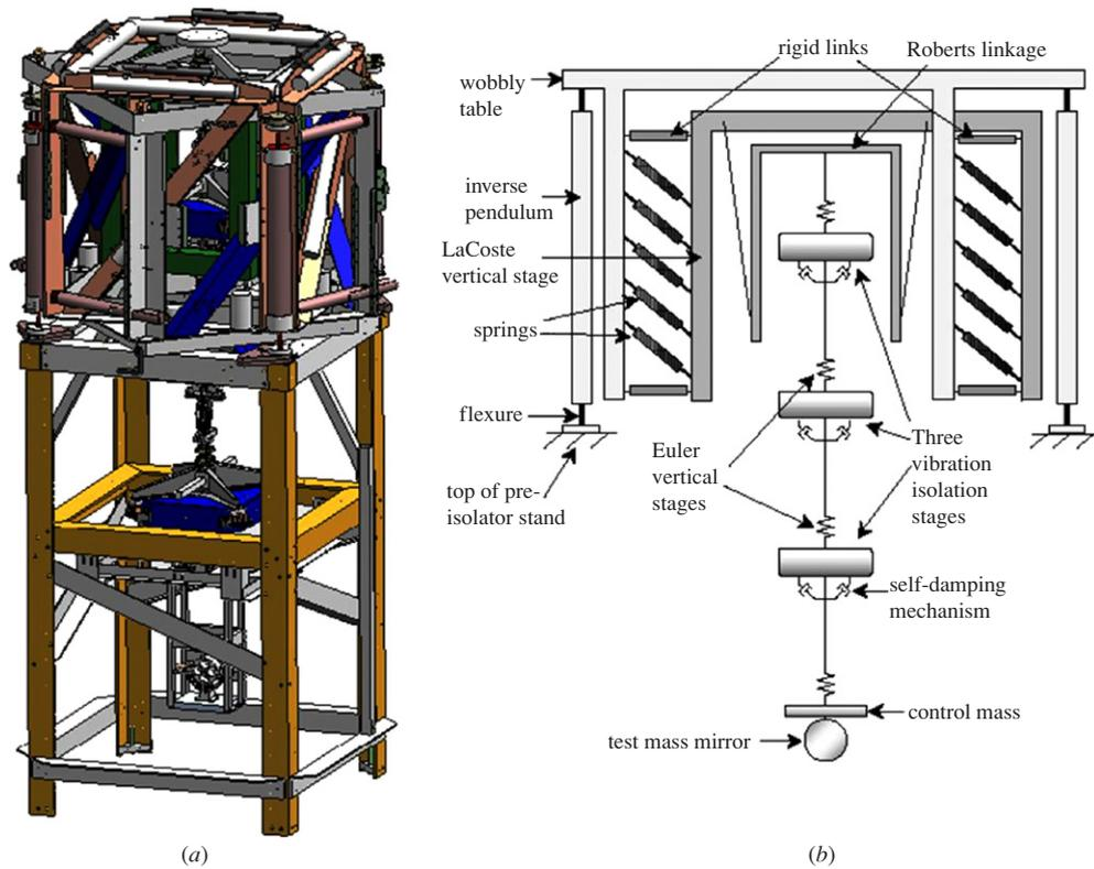
**Figure 2.** (a) Complete AIGO vibration isolation system with LIGO I suspension and test mass dummy as last stage. (b) Schematic diagram of the AIGO vibration isolation stack showing the three main sections: pre-isolation stage, multi-stage vibration isolation chain and the test mass.
