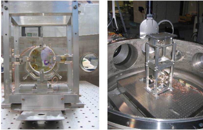
**Figure 5.** BK7 input test mass mounted on LIGO I suspension inside the tank just before closing it. The picture on the left was taken from the high reflection coating side, where it is possible to see the magnetic actuators behind the mirror.
